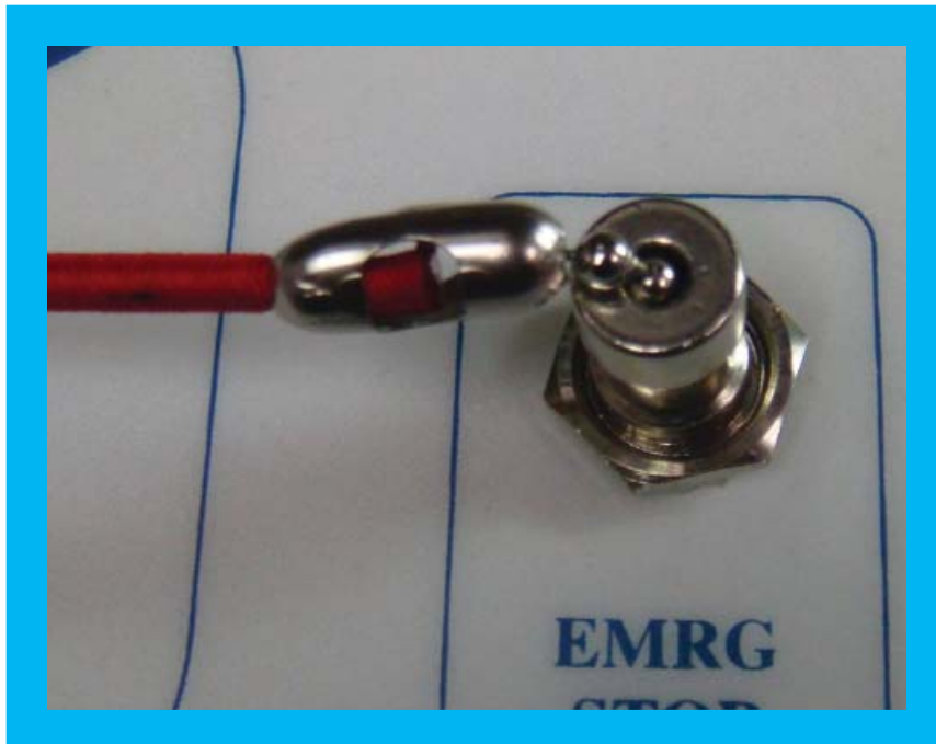
11.2 Install the emergency pull cord ball chain connector to the ball chain on the switch. Use pliers to crimp the two parts together.
