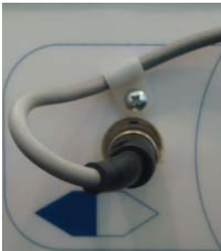
2.1 Remove hand controls crew
