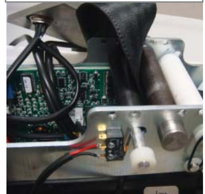
6.9 Remove both O-rings for the upper limit switch pin and pull out pin and roller.
